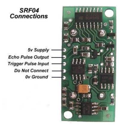
The S RF04 Timing diagram is shown below. You only need to supply a short 10uS pulse to the trigger input to start the ranging. The SRF04 will send out an 8 cycle burst of ultrasound
